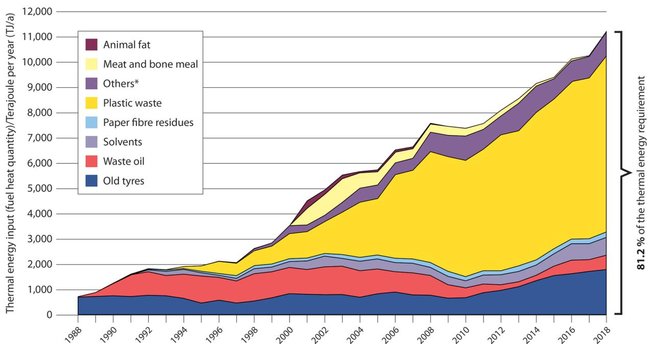
**Fig. 4:** Development of the recovery of secondary fuels in the Austrian cement industry: 1988 – 2018.
